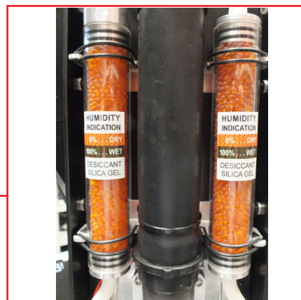
Silica gel desiccants in the fixture arm
